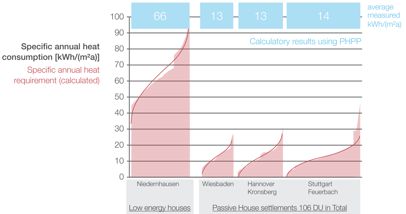
Figure 3: Overview of consumption measurements. This diagram summarises the measured heat consumptions from four housing estates, a low-energy settlement (left) and three Passive House settlements. [Passivhaus Institut, 2017]
